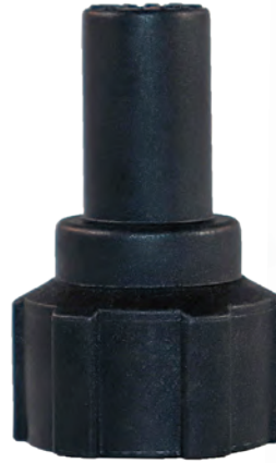
SE-RCAP-04P SE-RCAP-04PB Material: Valox Height: 2-3/16" Thread: 1-1/16"-18
