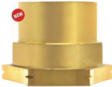
SE-RCAP-RB100 Material: Brass Height: 1-11/16" Thread: 1-7/8"-18 UNF Cap for WATTS Ball Valve RB100 Found on Kaiser Warren Racks between Suction Header and Accumulator.
