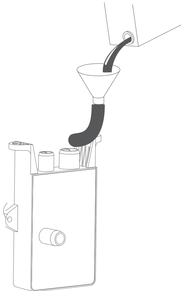
Fig. 49 – Priming Condensate TRAP (Appearance May Vary)
