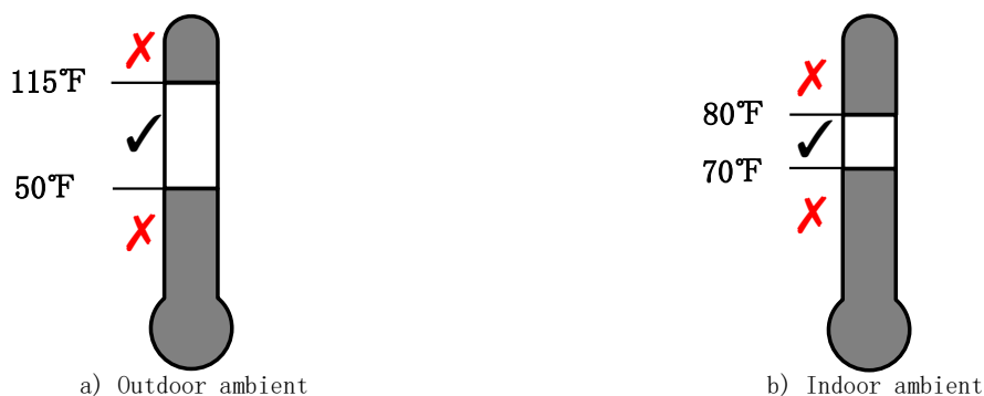
Figure 8.2 Temperature limit for AUTO charge mode
