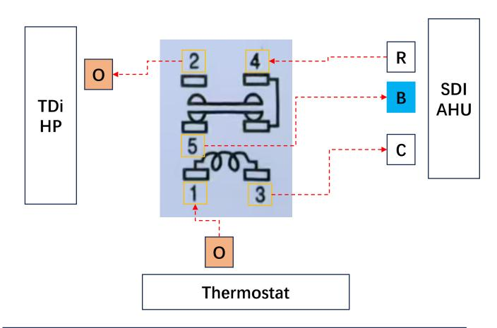
O/B conversion wiring diagram, the rest refer to conventional wiring.
