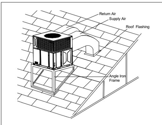
Figure 3.9 Rooftop Installation - Frame Mounting
