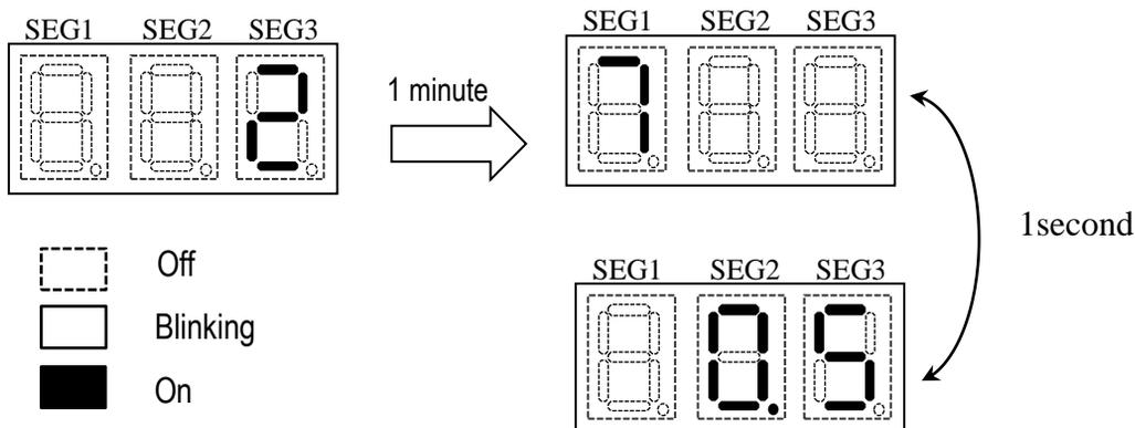
Figure 8.3 LED display in AUTO charge mode
