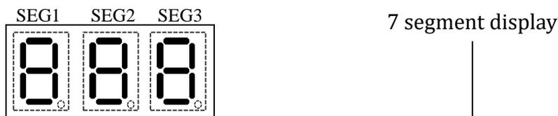
**SEG1:** Normally blank, but it displays codes “0 to 9” accordingly if there is damaged sensor and command response.
