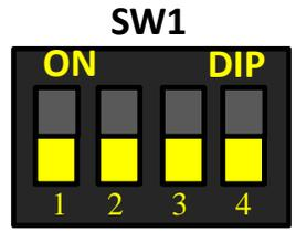
Use minor straight screwdriver to dip switch. Must power off the unit for at least two minutes to activate the change.
