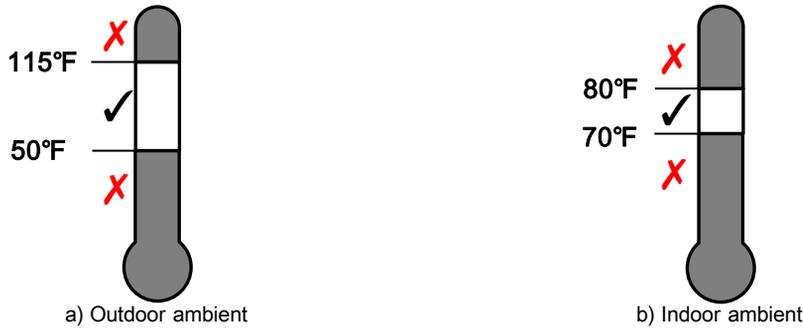
Figure 8.2 Temperature limit for AUTO charge mode
