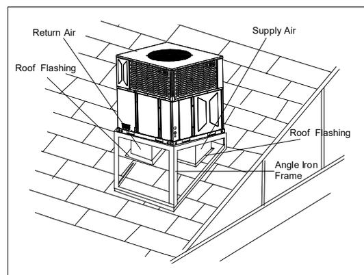
Figure 3.10 Rooftop Installation - Frame Mounting
