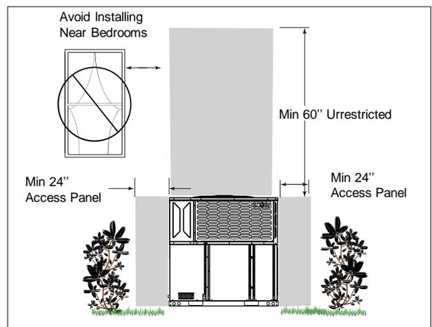
Figure 3.4 Clearance requirement
