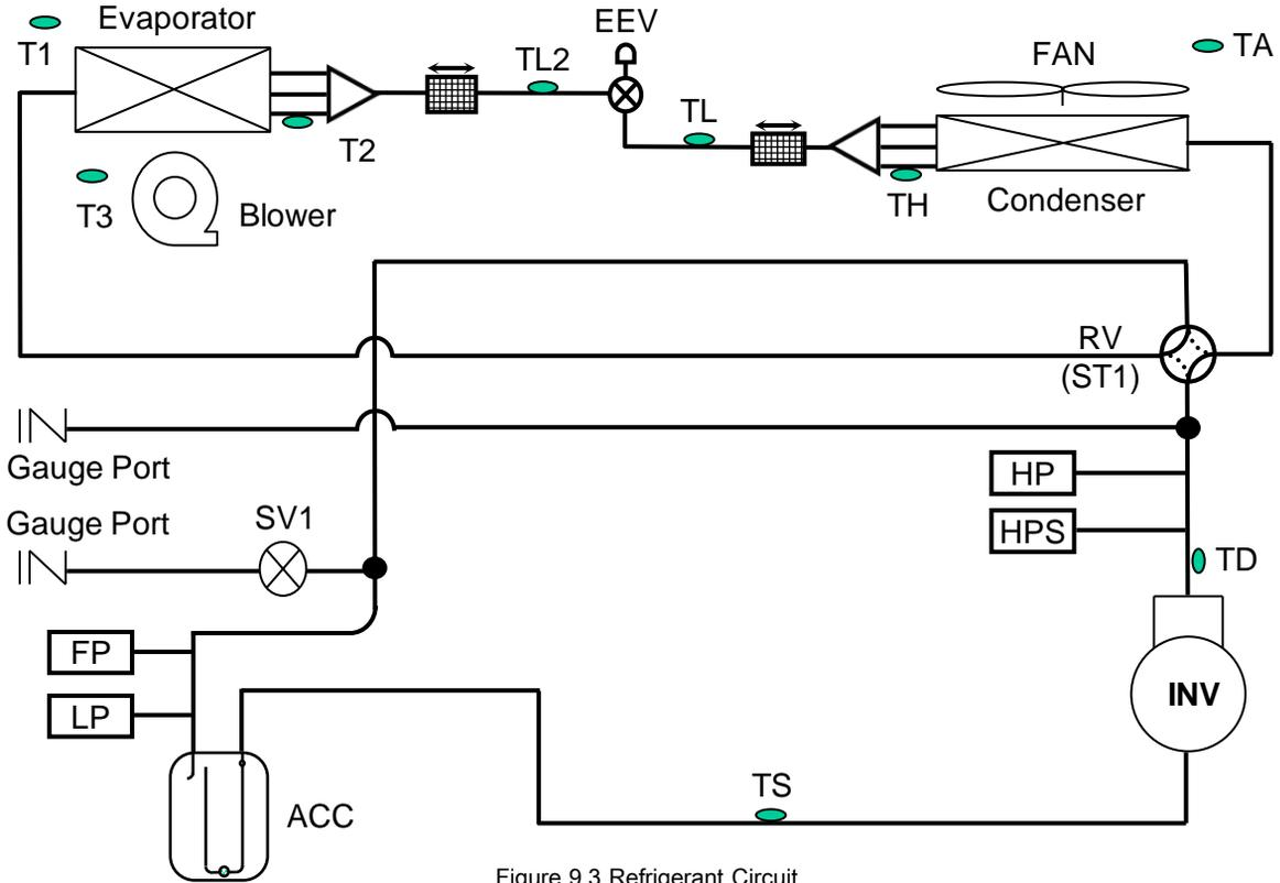
Figure 9.3 Refrigerant Circuit
