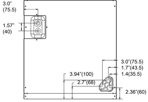
Figure 3-3 Dimensions for front connection coil
