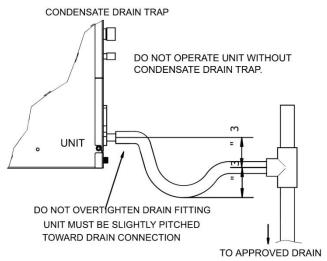
Figure 7-1 Condensate drain trap
