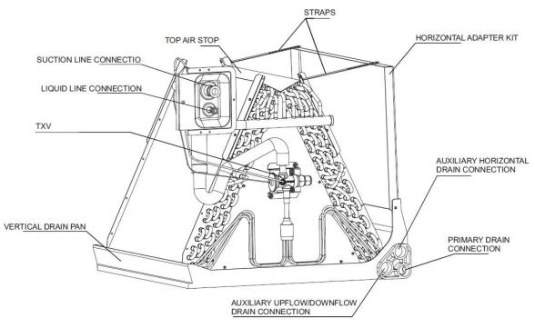
Figure 3-4 Evaporator coil
