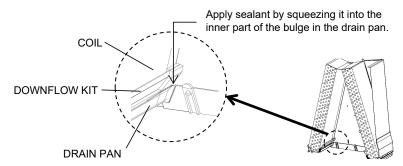
Step 3: Reassemble the coil back into the unit
