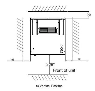
Figure 2-2 Clearance requirement
