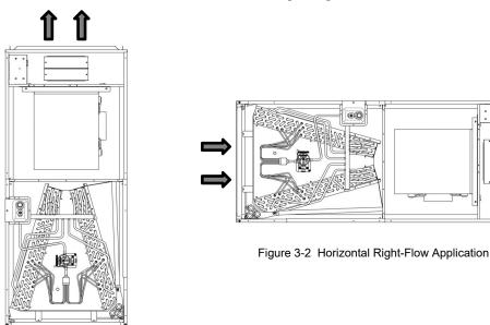
Figure 3-1 Vertical up-Flow Application
