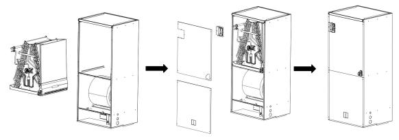
Horizontal left application: Simply install a Downflow Kit on the top, and apply sealant to the two corners of the drain pan and coil on the side where the Downflow Kit is installed.
