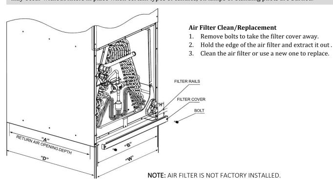
Figure 8-1 Filter installation and clean
