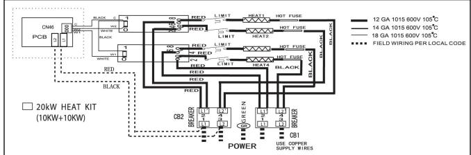
Figure 4-3 Wiring diagram for electric heat
