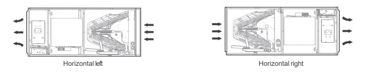
Note: Vertical up and horizontal left installation does not need to change the direction of evaporator.
