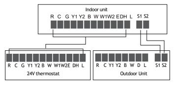
NOTE: The wiring method of the thermostat and the indoor unit refers to the wiring of the non-communication scheme.
