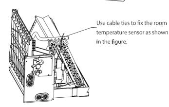
11. Reinstall evaporator cover plate.
