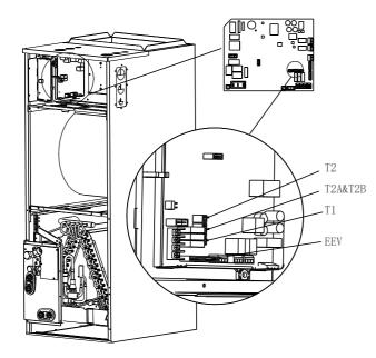
6. Take out the evaporator and drain pan and rotate 180°.
