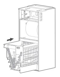
Note: The wire body needs to pass through the wire groove from the drain pan and be stuck on the hook of the drain pan. 10. The evaporator is assembled in place.
