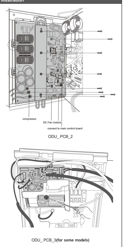
6) Remove the 1 screw and disconnect the wires and then remove the 24V board.(see ODU\_PCB\_3)(for some models)
