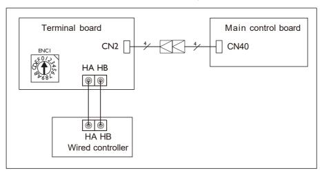
For some models: The wired controller connects to terminal board, terminal board connects to main control board.
