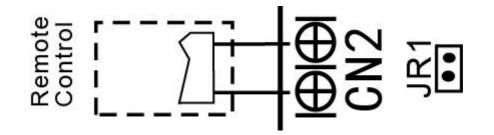
B.For remote control (ON-OFF) terminal port CN2 and short connector of JR1
