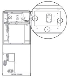
3. Install the electric auxiliary heating assembly into the chassis shell from the front, and note that the front end needs to be inserted into the shell assembly hole.
