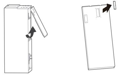
2. Remove the terminal block and power cord, loosen the screws, and remove the electric auxiliary heating cover.
