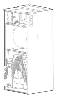
8. Reinstall the evaporator and drain pan.
