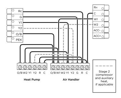
NOTE Do not connect any jumper wires between Rc and Rh. ecobee does this automatically. The R wire needs to go into the Rc terminal on your ecobee.
