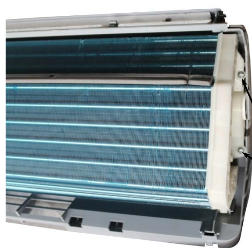
Two screws at the base bearing side
