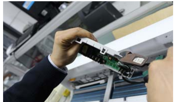
Fig. 28 — Cut a hole on the multi-function board
