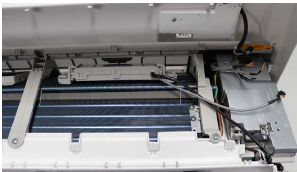
Fig. 32 — Connect the multi-function board
