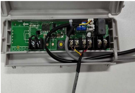
Fig. 30 — Connect the cable to the board
