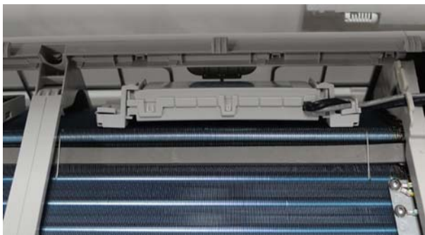
Fig. 31 — Install the multi-function board
