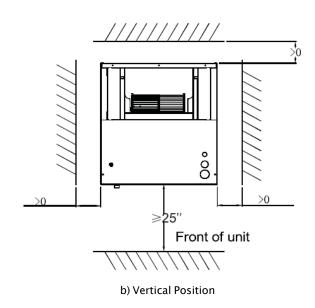
Figure 2-2 Clearance requirement
