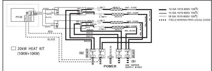
Figure 4-3 Wiring diagram for electric heat
