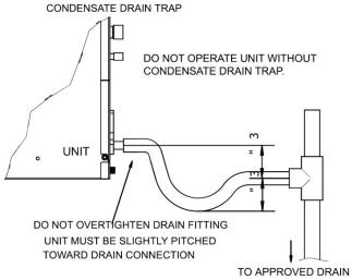
Figure 7-1 Condensate drain trap
