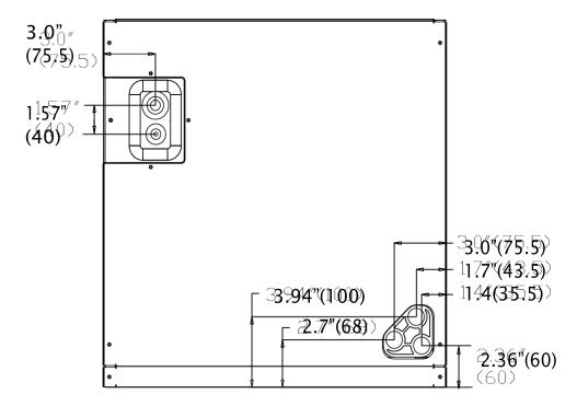
Figure 3-1 Dimensions for front connection coil
