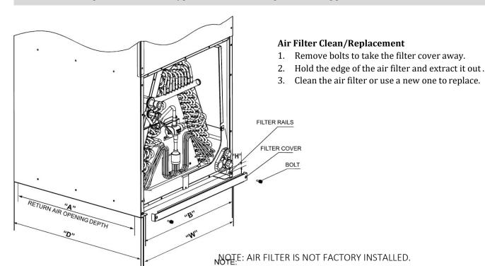
Figure 8-1 Filter installation and clean
