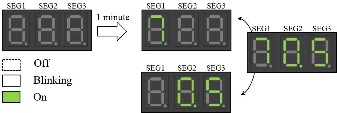
Figure 13-1 LED display in AUTO charge mode
