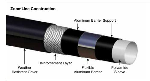
**ZoomLine** has been designed to eliminate refrigerant leakage while maintaining flexibility not available with copper tubing. The 6 layer hose is designed to withstand environmental, temperature and pressure extremes while providing excellent installation flexibility and long life.
